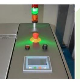
We have 3 cycles – washing with chemcial agent, rinsing with high pressured water and drying with pressured air. All 3 cycles are fully automatic and you only have to push one botton to start the machine. When the procedure is done – the machine shows an optical signal to understand that it is ready for the next roll. Of course you can programm cleaning and cycle times depending on the situation with each anilox.
